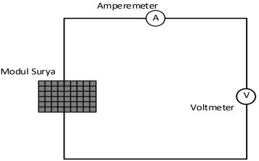
Figure 5. Schematic Figure of the Unloaded Solar Module Testing Circuit
