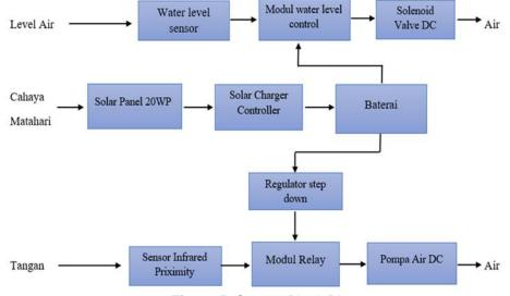
Figure 5. System Block Diagram
