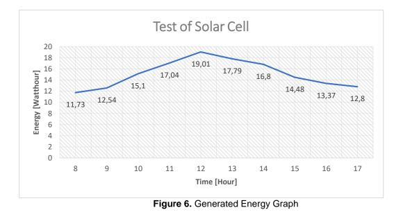
From the graph above, it can be seen that the greatest energy is generated at 12.00 with a voltage on the solar panel of 13.87 Volts and a current of 1.37 Amperes.
