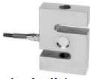
Figure 4. Load cell type S (Kurnia et al., 2019)
