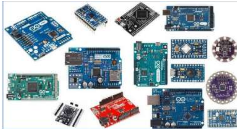
Figure 2. kinds of arduino micro controllers (Ismailov & Jo'rayev, 2022)
