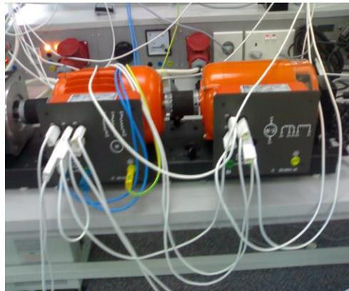
**Figure 6.** Wiring of Induction Motor Couple DC Motor
