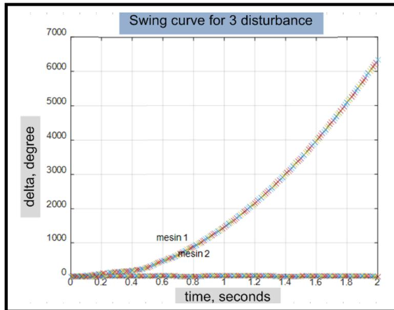
**Figure 10.** Graph of Delta Simulation Results Against Time on Transmission Lines 3-4 Near Bus 4. Interruption Termination Time 0.23 seconds S
