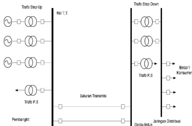
**Figure 1.** Schematic of the Electric Center Connected Through the Transmission Line to the Load (James A. Pongtiku, 2014)
