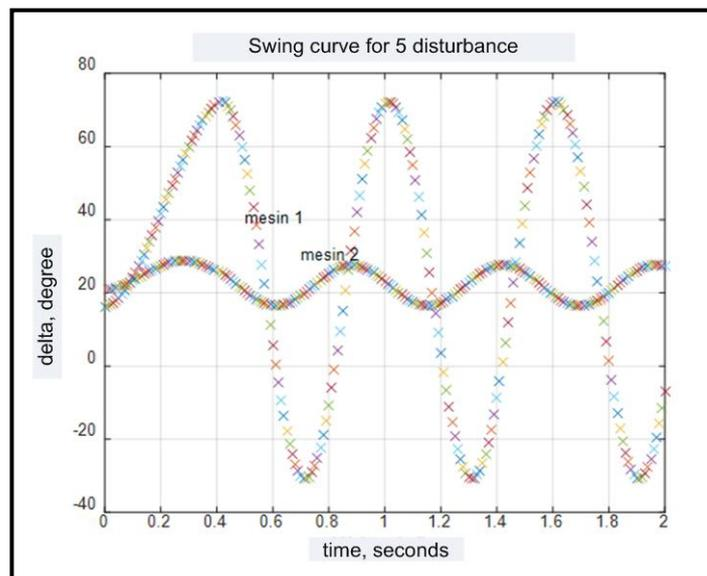
**Figure 13.** Graph of Delta Simulation Results Against Time in the Middle of Transmission Line 5-3(2). Disconnection Time 0.4 Seconds
