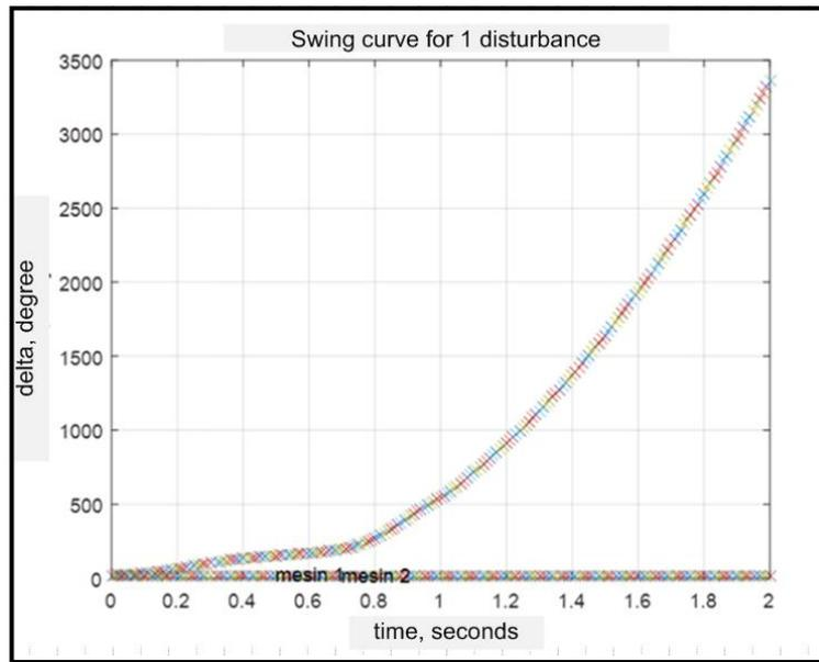
**Figure 6.** Graph of Delta Simulation Results Against Time on Channel 3-4 Near Bus 3, Disconnection Time of 0.3 Seconds
