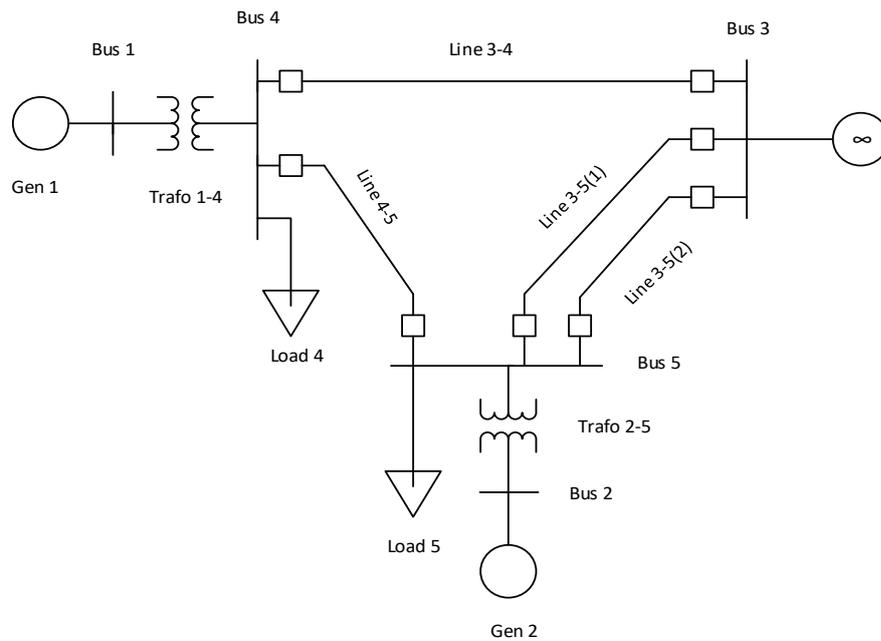
**Figure 3.** Single Line Diagram of a 5 Bus 2 Generator System
