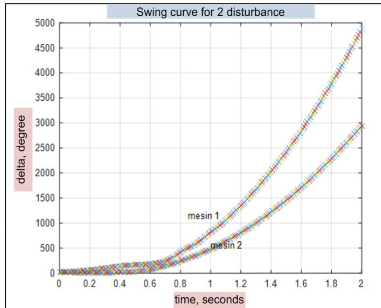
**Figure 8.** Graph of Delta Simulation Results Against Time in Transmission Line 3-5(1). Disconnection Time 0.39 Seconds
