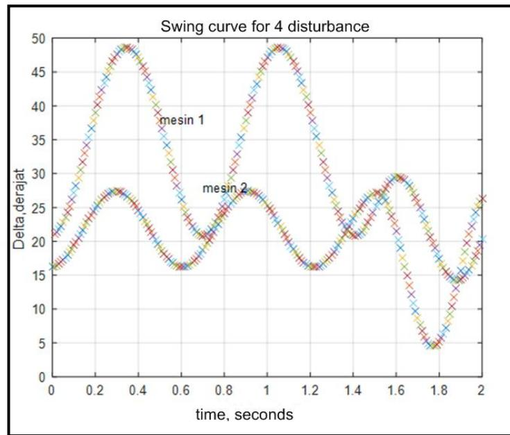
**Figure 12.** Graph of Delta Simulation Results Against Time in the Middle of Transmission Line 4-5. Interrupt Termination Time 1.5 Seconds
