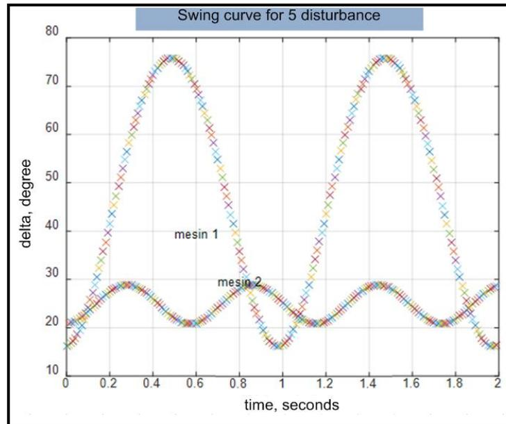
**Figure 14.** Graph of Delta Simulation Results Against Time in the Middle of Transmission Line 5-3(2). Interrupt Termination Time 2 Seconds
