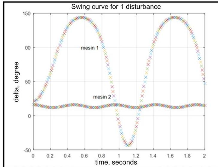
**Figure 5.** Graph of Delta Simulation Results Against Time on Transmission Lines 3-4 near bus 3, Disconnection Time 0.29 seconds
