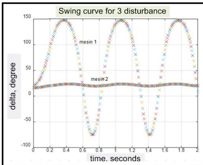
**Figure 9.** Graph of Delta Simulation Results Against Time on Transmission Lines 3-4 Near Bus 4. Interruption Termination Time 0.22 Seconds
