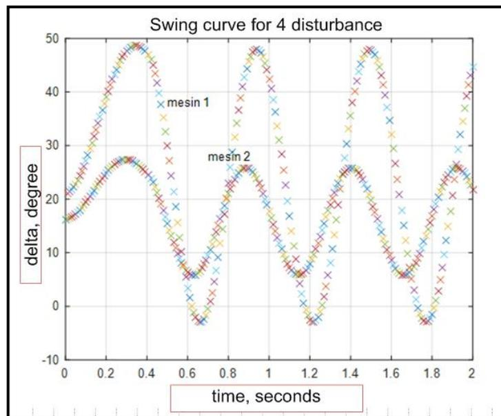
**Figure 11.** Graph of Delta Simulation Results Against Time in the Middle of Transmission Line 4-5. Disconnection Time 0.4 seconds
