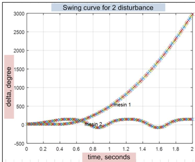
**Figure 7.** Graph of Delta Simulation Results Against Time on Transmission Lines 3-5(1) Near Bus 3. Disconnection time of 0.38 seconds
