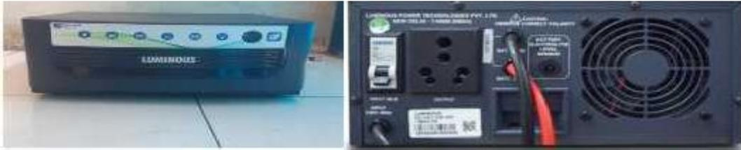
Gambar 6 Inverter Sine Wave UPS Luminous 1000 watt/12VDC/220VAC
